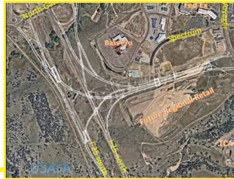
Detail of the new Powers-Voyager I-25 interchange to be south of the North Gate interchange
